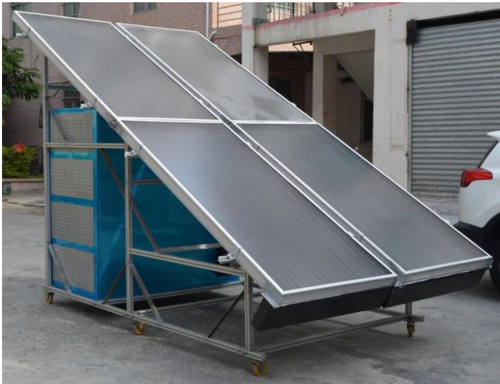
Each group of four solar air collectors is matched to dual blower fans, ductwork and a cabinet with 4 compartments and 24 drying racks, each approximately 1 square meter, so that approximately 60 KG of wet fruit can be dried at one time. By simply adding modules this can be multiplied depending on the capacity required.
