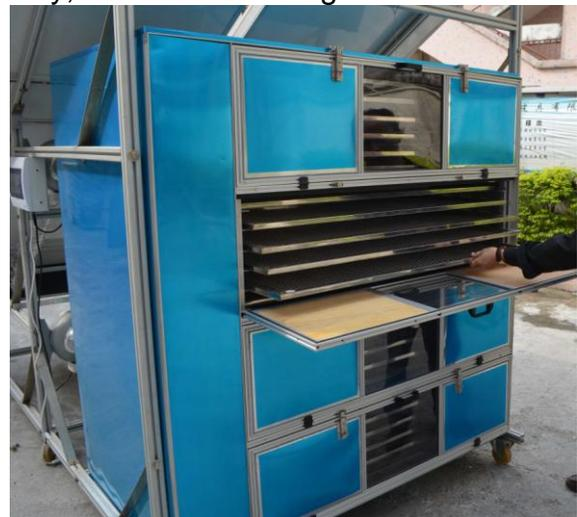
This SolarFlex Quad system, like the “Small Farm” model, employs the high-performance horizontal airflow method through the cabinets and drying racks. This method, though slightly more complex, has been scientifically proven to be superior to typical vertical airflow systems. Horizontal airflow allows the drying air to sweep across the surface of the food (including the “boundary layer”) which is much more efficient than pushing up air against the bottom of the food.
